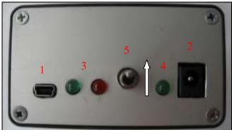
Controller front; switch in NORMAL position
