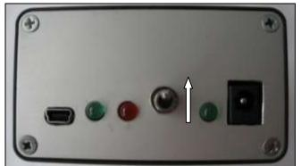
Controller front; switch in NORMAL position
